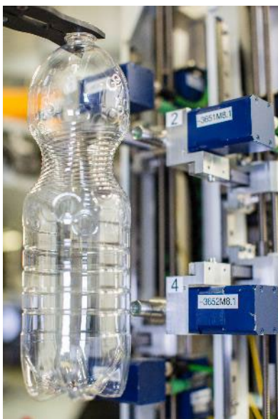
Figure 1 above shows how high-precision wall thickness measurements are taken at the most representative points of each bottle, using four interferometric sensors based on reflected infrared light.
