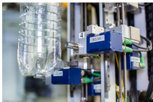
Figure 1 above shows how high-precision wall thickness measurements are taken at the most representative points of each bottle, using four interferometric sensors based on reflected infrared light.
